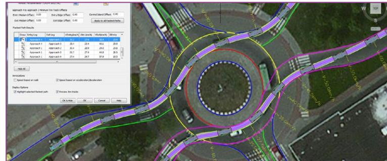
Vehicle speed analysed on a custom drawn roundabout, providing vital input for improving traffic safety.
